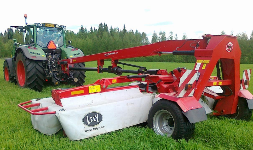
TRIAL 1. Topping at the height of 30 cm by Lely Splendimo 550 P disc mowing machine.
