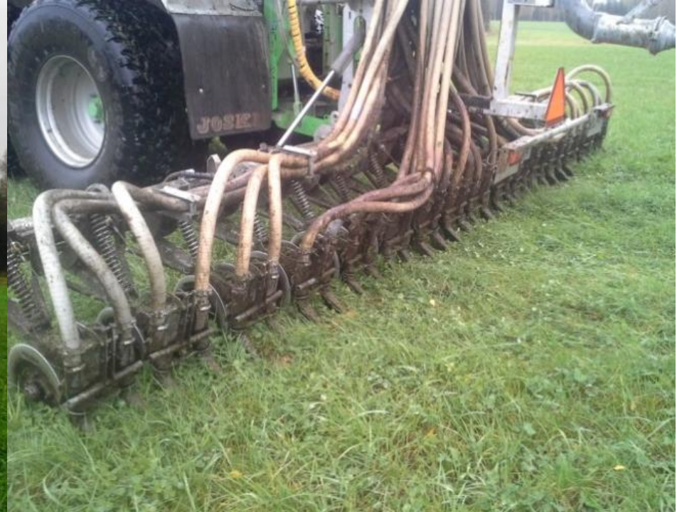
TRIAL 2. The slurry was injected directly into the sward by Joskin slurry tanker.
